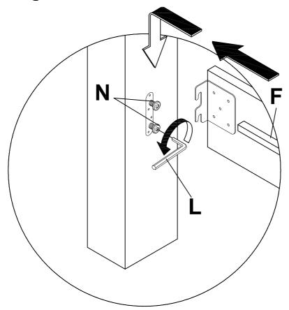
STEP 4 Attach the side rail (F) to footboard (D) by pushing the bracket down to fit it
