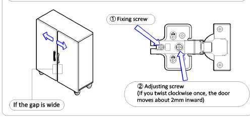
• There is a gap on the top of the door when doors are closed (Glass slide hinge does not require this step) (4 screw hole hinge does not require ①)
