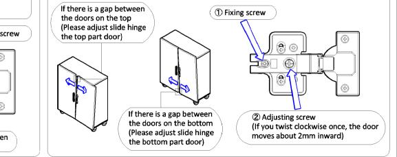
There is a gap on the top of the door when doors are closed (Glass slide hinge does not require this step) (4 screw hole hinge does not require ①)
