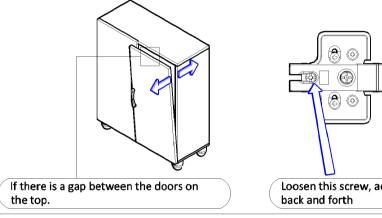
Loosen this screw, adjust by moving
