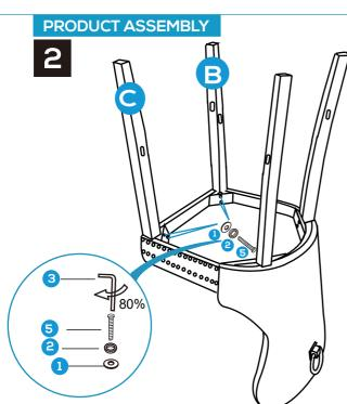
Align front legs in the seat pad as shown in the diagram.
