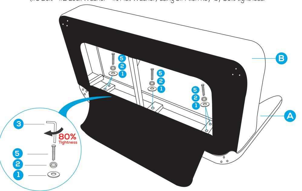
Attach Part C Leg to Chair Bottom with 12pcs Hardware 6# Bolt using 4# Allen Key
