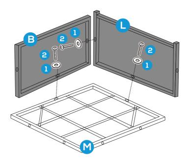
Attach the assebled part (B+L+M) to part A Corner Right Side and part N Corner Left Side with 6 PCS of part 1 washer and part 2 bolt.
