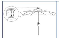
**Step 1:** Insert the plug into the socket under the solar panel. Then, insert the bottom pole into the umbrella frame
