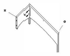
STEP 10 Connect the part from step 9 and table side frame H with bolt N with allen key
