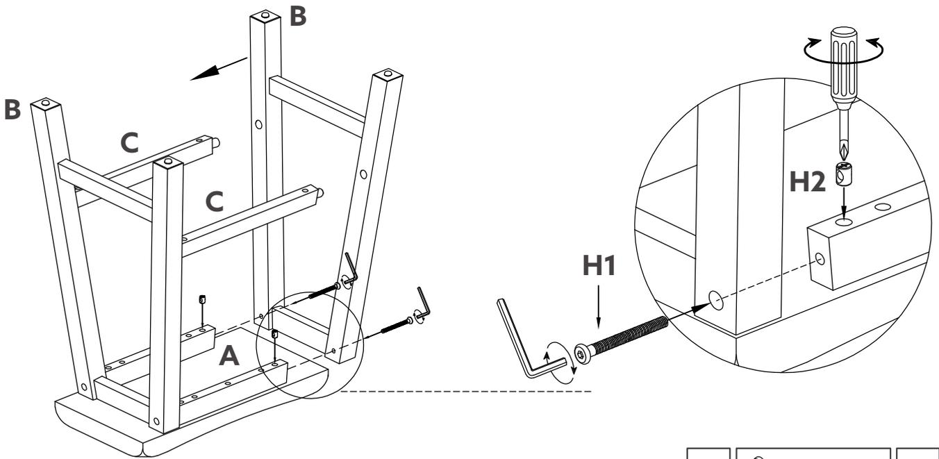
Be sure the legs are level then fully tighten the leg bolts
