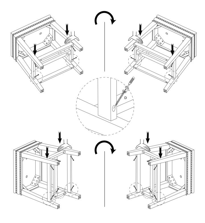
Press the legs and stretchers to make sure no gaps then tighten the screws.
