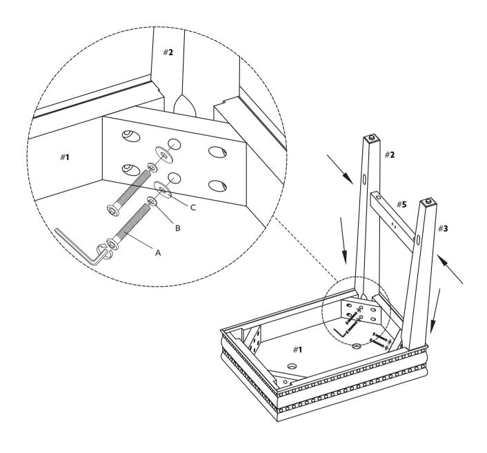
Do not tighten bolts completely until all bolts are completely lined up and inserted into holes.
