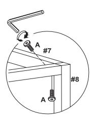
Do not tighten bolts completely until all bolts are completely lined up and inserted into holes.
