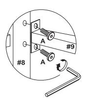
Do not tighten bolts completely until all bolts are completely lined up and inserted into holes.
