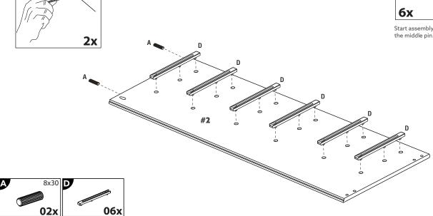
Attention! Do not use nails or screws to secure the glides to the side panels. A soft beat with a hammer in the correct sequence is enough.
