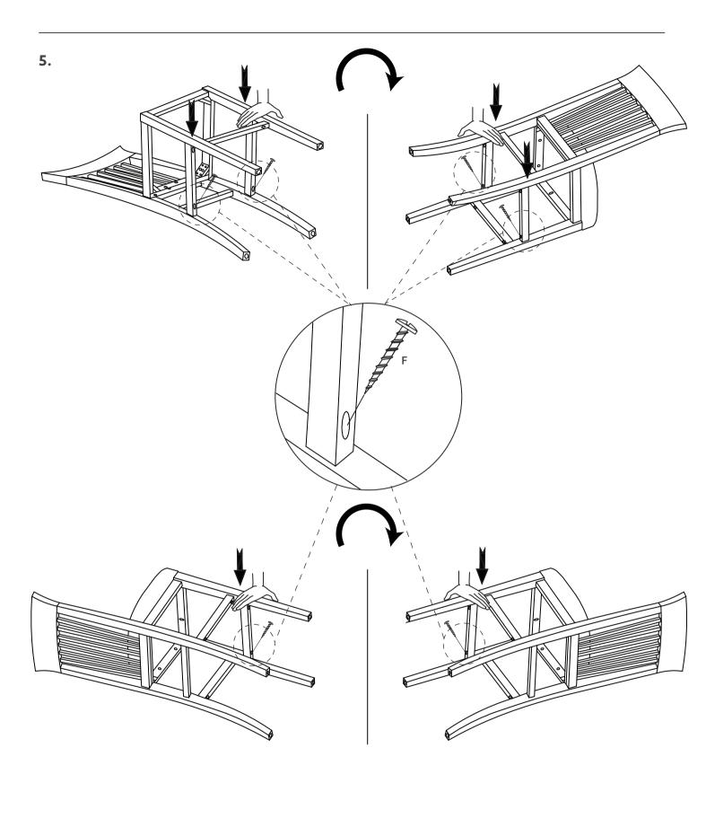
Press the legs and stretchers to make sure no gaps then tighten the screws.
