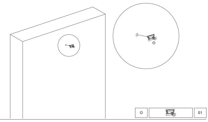
PLEASE NOTE: For your safety, to prevent the danger of this unit tipping over, it is important that the wall anchors are properly attached.
