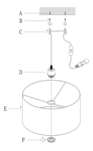
CAUTION: Once being mounted, do not pull on lamp as this may cause injury to persons and damage to the lamp and mounting surface. To reduce risk of such injury or damage, mount on a surface that is mechanically solid. Fasten mounting hardware to wooden ceiling support beams only. Do not mount to plasterboard.
