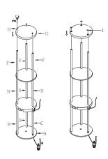
Place shade (L) onto the socket, then screw the socket ring (M)
