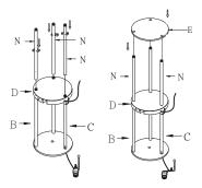
4. Screw all 3 poles (F) one by one into 3 poles (N) through thin shelf (E) to tighten.
