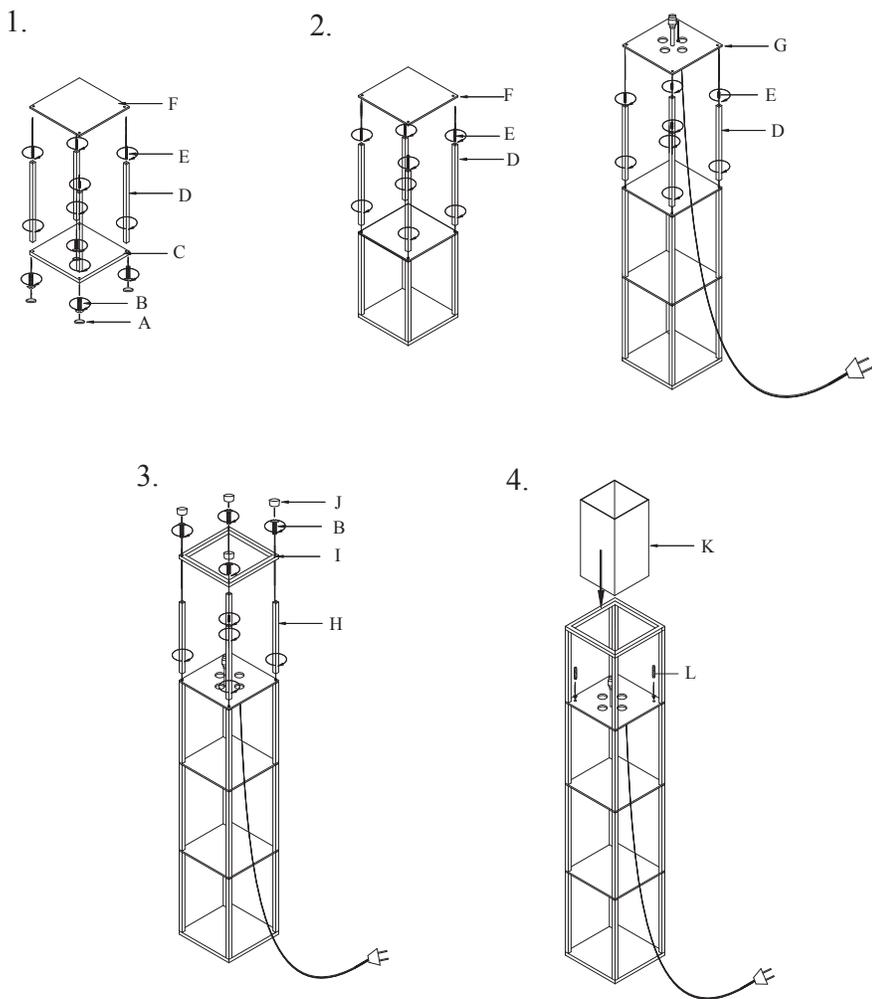
1. Assemble PART (C) and PART (F) with PART (D) and fasten with PART (A) and (B).
