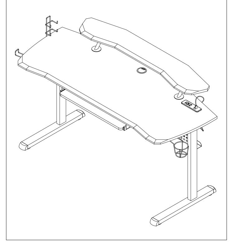
\*\* Do not fully tighten screws until fully assembled \*\*\*
