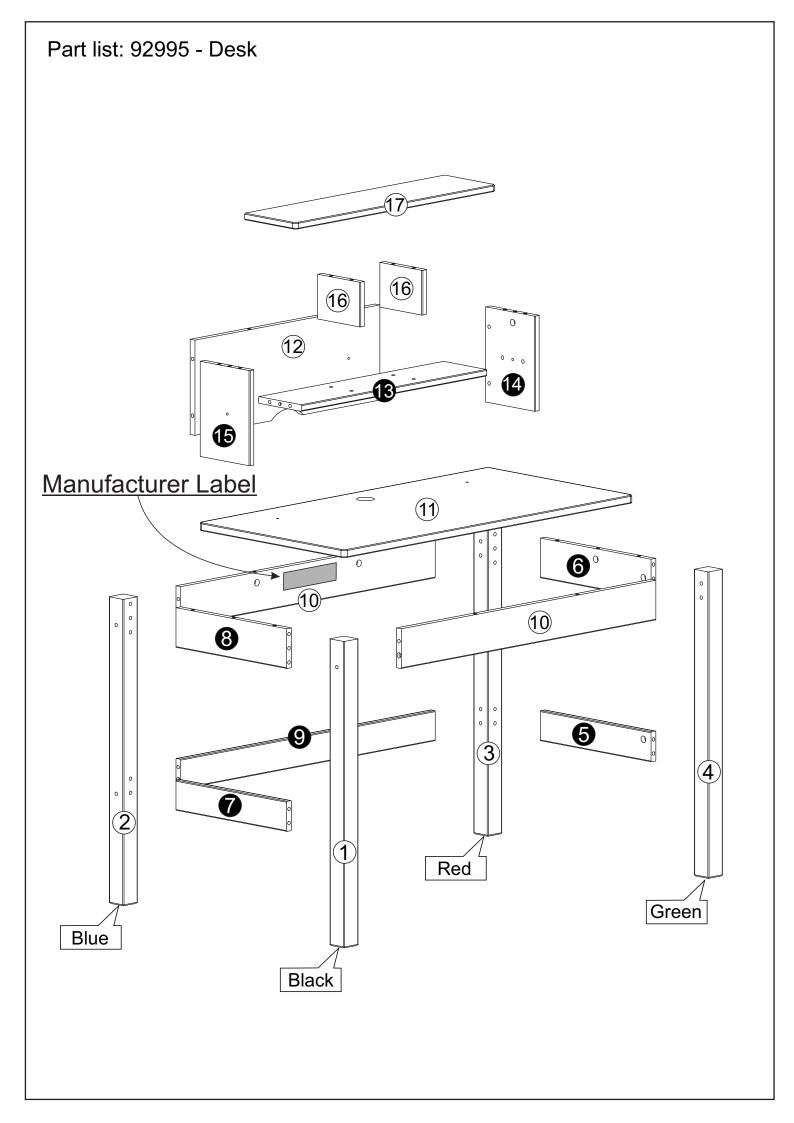
**Identifying the Hardware/part list** - Identify the hardware using the illustrations below.
