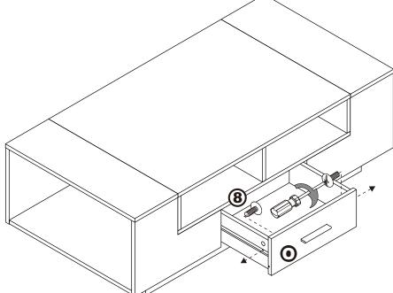
Extend the two outer slides of the runners so that they could align with the sides of the drawer. Make sure the pre-drilled holes from the drawer align with the screw holes of the outer slides. Secure two screws from the inside of the drawer using a Phillips screwdriver to tighten them to the outer slides.
